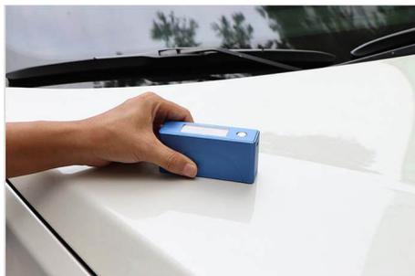
**MetriTec™ Gloss Meter M193** is a portable gloss meter with micro measuring aperture, universal angle 60°. Its measuring range is 0-1000GU, and exclusively applicable to surface gloss measurement on curved or mini size material.
