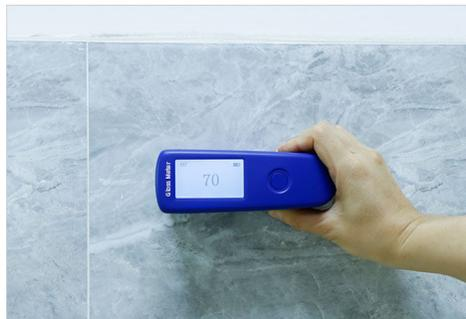
**MetriTec™ Gloss Meter M192** is a hand-held gloss meter with universal measuring angle 60° and its measuring range is 0-1000GU. The instrument is widely used in surface gloss measurement on paint, coating, metal, ceramics, stone, printed material. It's so convenient that you can use even without pressing button. QC mode is optional to conduct quick QC process. Intelligent data statistics and test report can be generated by connecting PC software.
