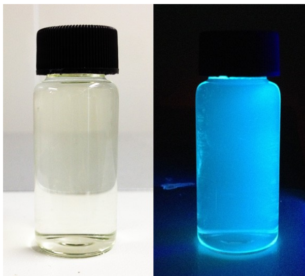
Emission photos (1) of ACS Material Blue Luminescent Graphene Quantum Dots excited by Natural light(left) and UV light(right)
