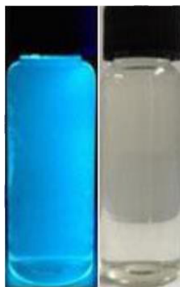
Fig.1 Photos of Blue Luminescent Graphene Quantum Dots Powder at 365 nm UV lamp (left) and under natural light (right)
