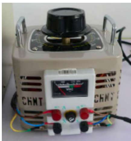
Photo of Voltage Regulator
