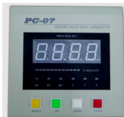
Photo of Digital Pulse Modulator Panel
