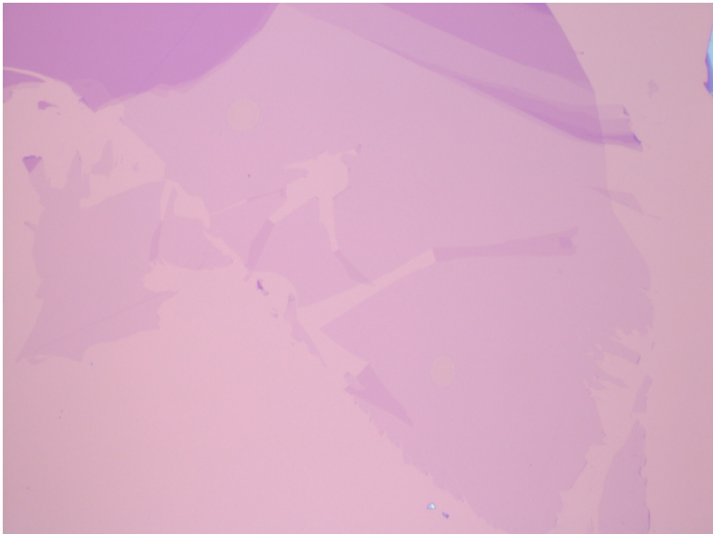
Typical Image of ACS Material Mechanically Exfoliated Bilayer Graphene on 300nm SiO 2
