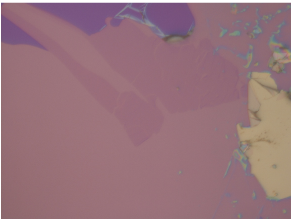
Typical Image of ACS Material Mechanically Exfoliated Monolayer Graphene on 300nm SiO 2
