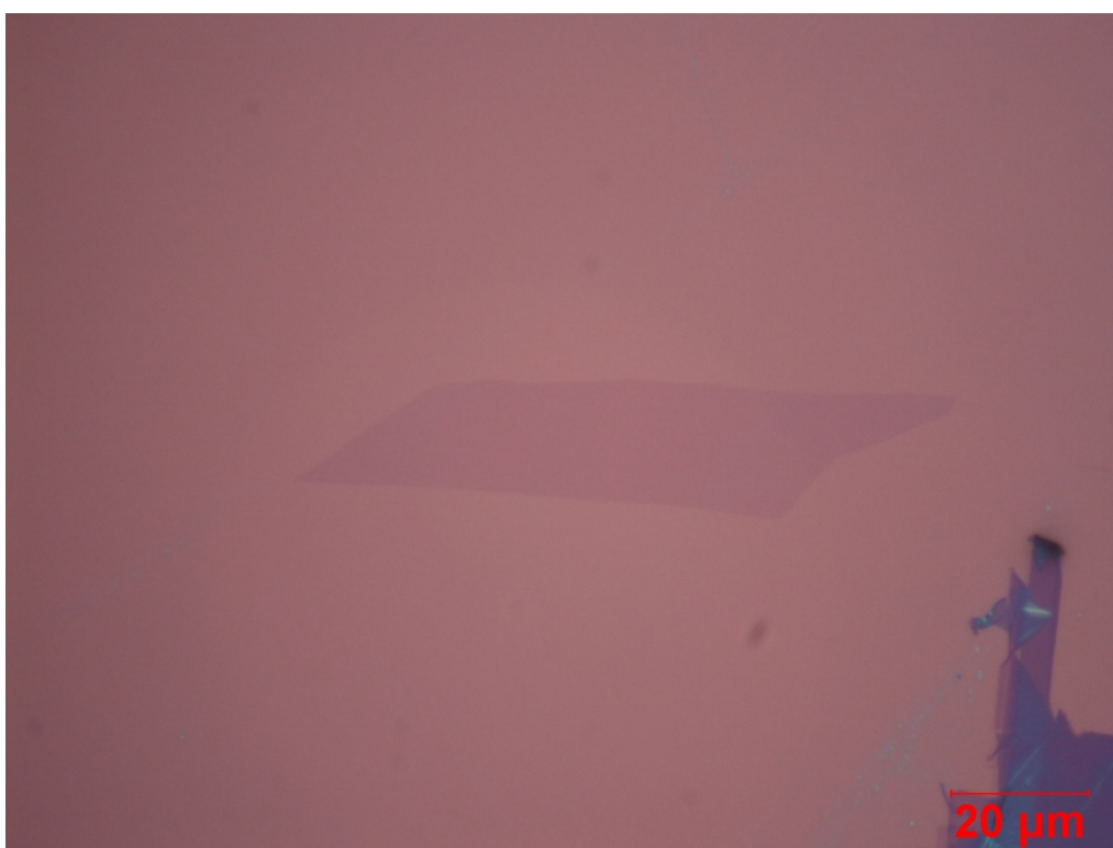
Typical Image of ACS Material Mechanically Exfoliated Monolayer Graphene on 90nm SiO 2
