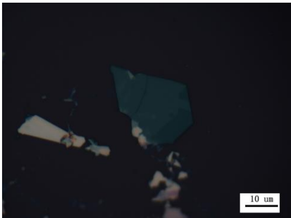
Typical Image of ACS Material Mechanically Exfoliated Monolayer MoS 2 on SiO 2 substrate
