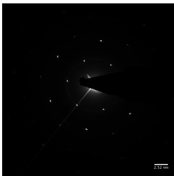
Typical Crystal Diffraction Image of ACS Material Monolayer TTh-BN
