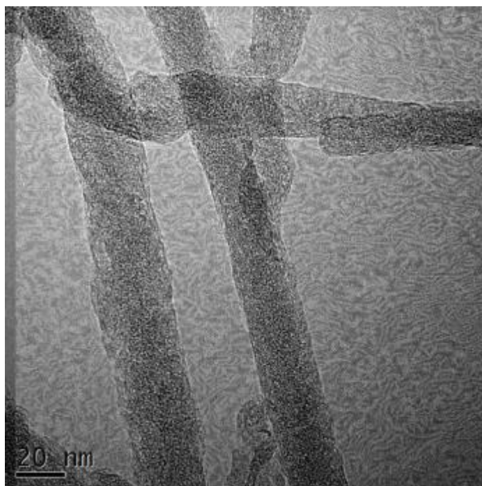
Typical TEM Image of ACS Material Fluorinated Carbon Nanotubes
