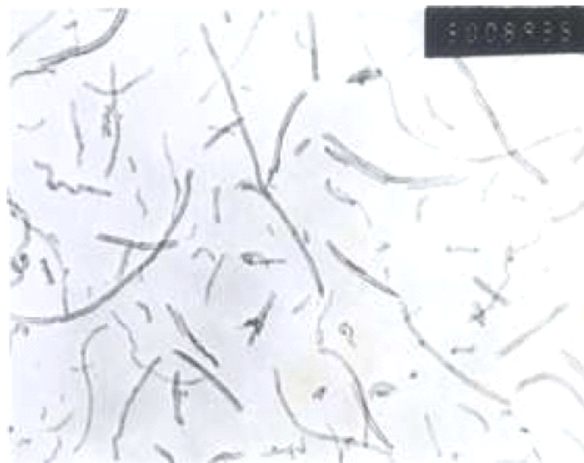
SEM Image (1) of ACS Material Purified MWNTs-COOH (Length = \sim 50 \mu\text{m} )
