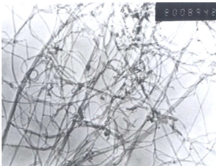
SEM Image of ACS Material Purified MWNTs-COOH (Length = 10-30 \mu\text{m} )
